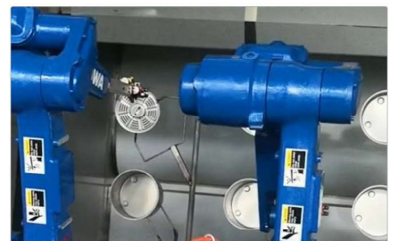
Robot kitchenware spraying project
