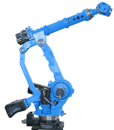
ALPHTIC Series Payload : 500kg
