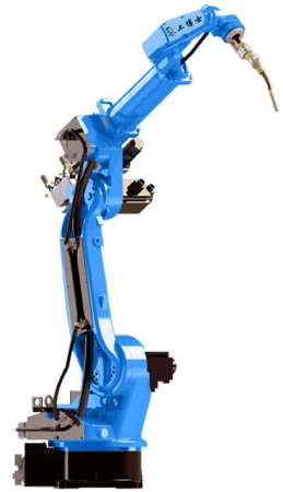
ARC Series Payload : 6kg
